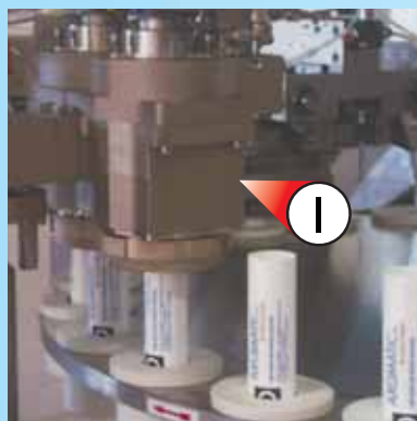
GRUPPO ARIA CALDA PER TUBETTI IN POLITENE E LAMINATO HOT AIR SYSTEM FOR PLASTIC AND LAMINATED TUBES
